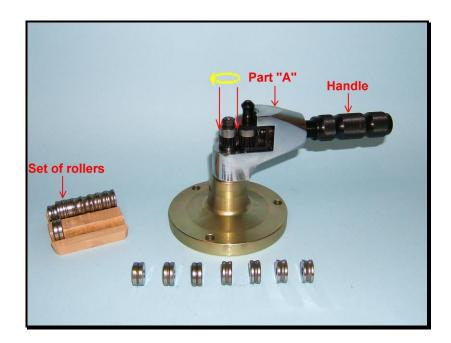
Our ringstretcher easily enlarges gem-set rings without the removal of the stone. It comes with a set of 16 dies in a plastic storage box + 2 already mounted on the stretcher.
